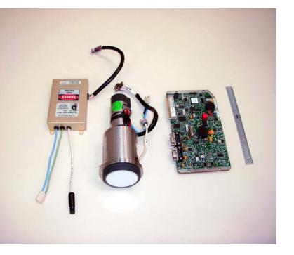
Palomar Display Products offers a ruggedized, militarized, highly reliable one inch miniature CRT with compact electronics that require less than 15 watts of power.
