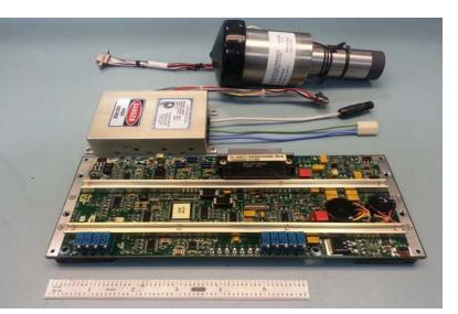
Palomar Display Products offers a ruggedized, militarized, highly reliable one inch miniature CRT with compact electronics that require less than 15 watts of power.
