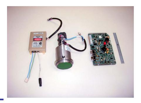
Palomar Display Products offers a ruggedized, militarized, highly reliable one inch miniature CRT with compact electronics that require less than 15 watts of power.
